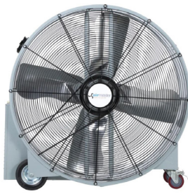
115V, 1 phase, 2 speed, ODP 1 HP motor #2595-60002 $490.10
